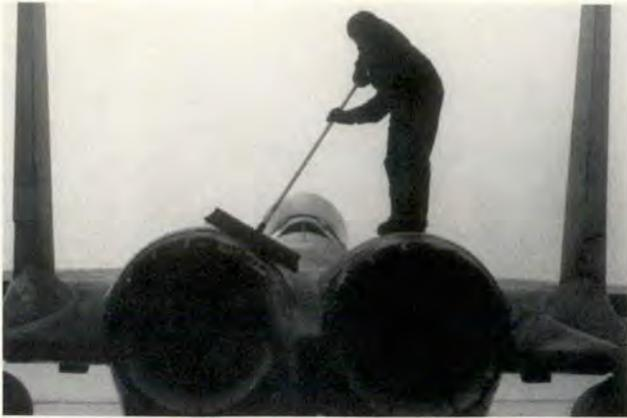
Sweeping snow off the aircraft before it melts and turns to ice saves time and deicing fluid.
