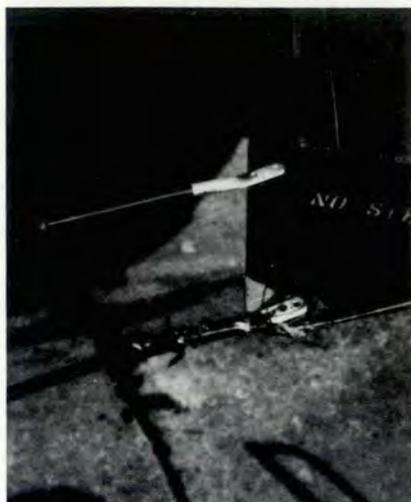
Designed to dissipate static buildup on aircraft, these "whiskers" were unable to handle the tremendous surge of a lightning strike.
