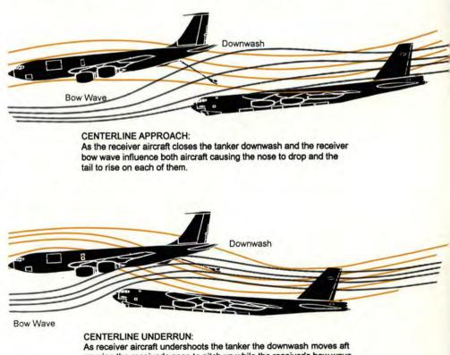
As receiver aircraft undershoots the tanker the downwash moves aft causing the receiver's nose to pitch up while the receiver's bow wave pushes the tanker's tail up.
