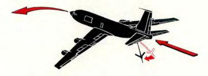
BOOM TURN: Swinging the refueling boom 8 degrees to the left or right of the centerline with the controls neutralized causes the boom to act as a rudder and will turn the aircraft towards the side the boom is moved.
