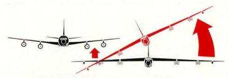
LATERAL UNDERRUNNING: Because of the changing angle of attack caused by the downwash off the tanker's wing, the receiver's wing under the tanker generates less lift while the receiver's wing in the free air generates more lift. The receiver aircraft will, unless corrected, roll up towards the tanker. of interrelated aerodynamic effects."
