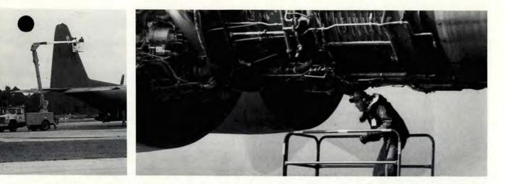
contributed to inadequate torque on pylon bolts due to severe space limitations to access the bolts. Working with Sacramento Air Logistics Center, McClellan AFB, California, a new torque wrench extension was designed, developed, tested, and approved. The results were significant fuel shop man-hour savings and a projected savings of \$1.2 million over a 5-year period.
