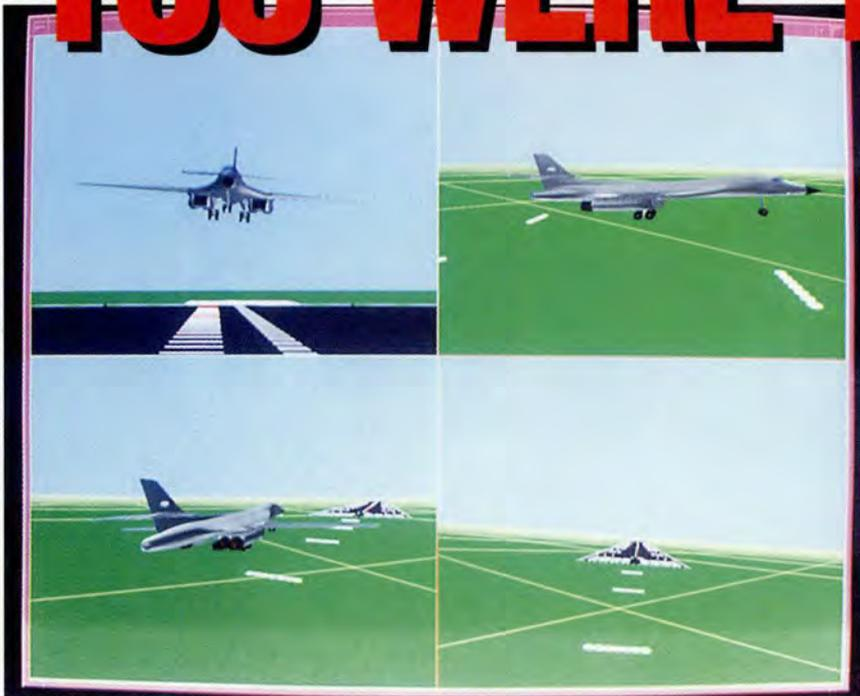
Once the recorder data and terrain information is loaded in the computer, animations of any portion of the flight can be viewed in real-time, fast or slow motion, forward or reverse.
