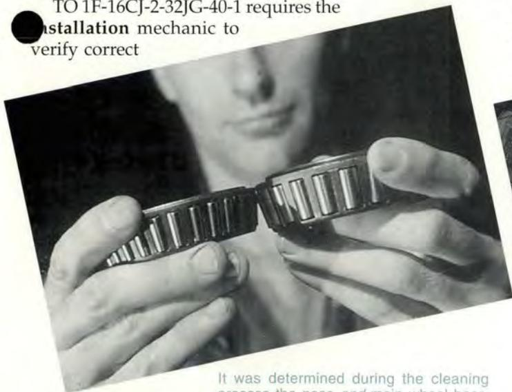
It was determined during the cleaning process the nose and main wheel bearings were "mixed" by shop personnel. However, the mixed bearings were supposed to be separated when they were repacked with grease
