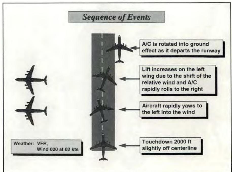
This graphic provides a notional representation of the aircraft's movements during the loss of control experienced by the aircrew.
