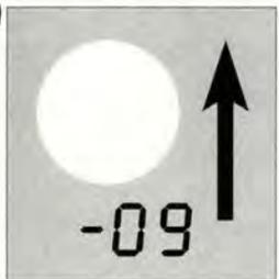
A symbol change to a filled yellow circle indicates that the intruding aircraft is considered to be potentially hazardous. Depending on your altitude, TCAS II will display a TA when the time to CPA is between 35 and 45 seconds.
