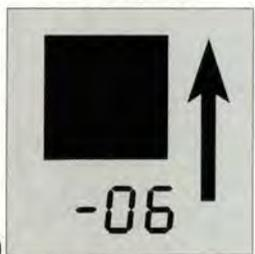
A solid red square indicates that the intruding aircraft is projected to be a collision threat. TCAS II calculates that the intruder has reached the point where a resolution advisory is necessary. The time to closest approach with the intruder is now between 20 and 30 seconds, depending on your altitude. The symbol appears
