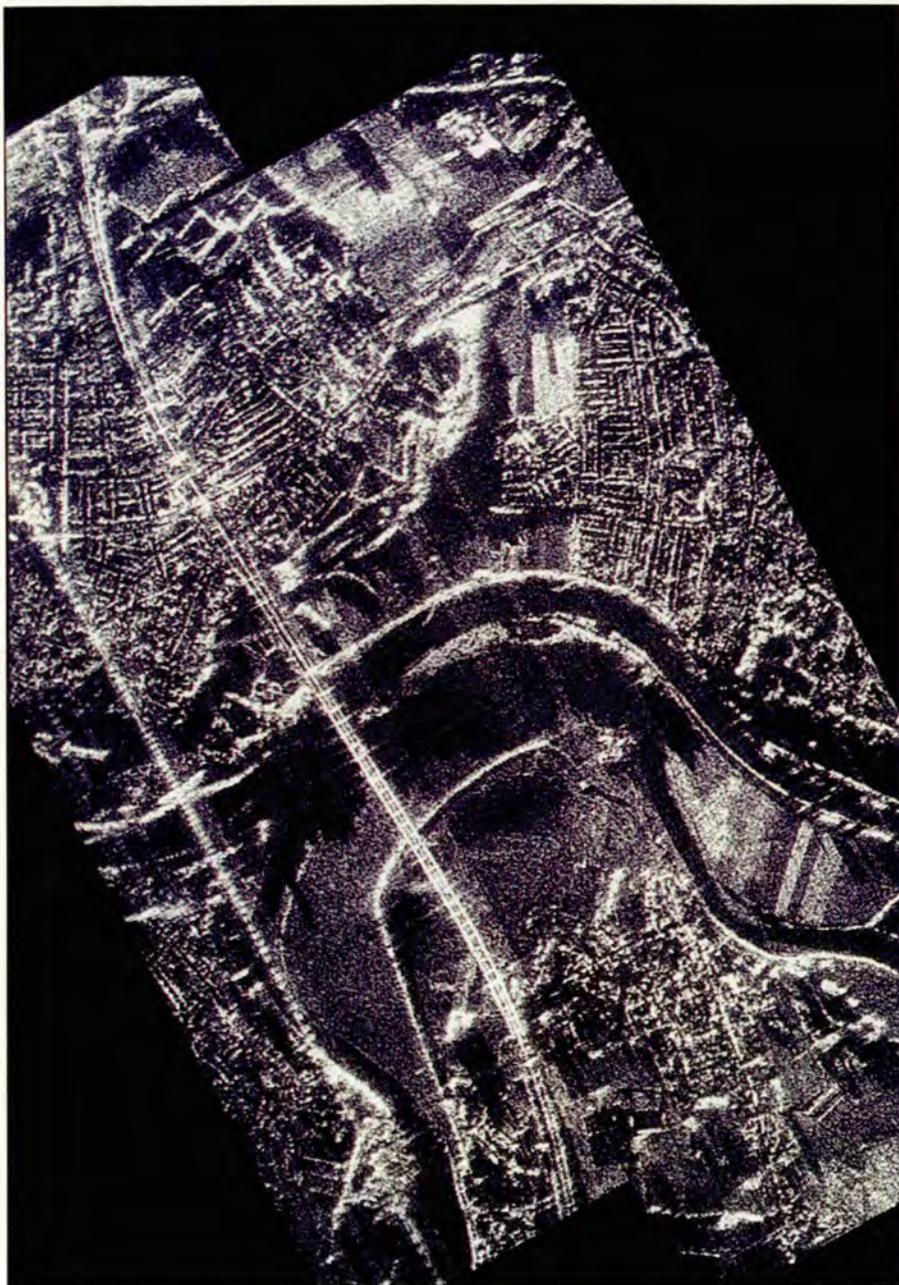
No bridge too far: The Rhine River and the surrounding countryside is clearly shown winding its way through Germany in this picture of the Joint STARS Synthetic Aperture Radar (SAR) mode. This mode furnishes imagery of land features, along with mobile targets that have become stationary, providing CSAR-dedicated forces with details concerning the terrain where downed crewmembers may be located.
