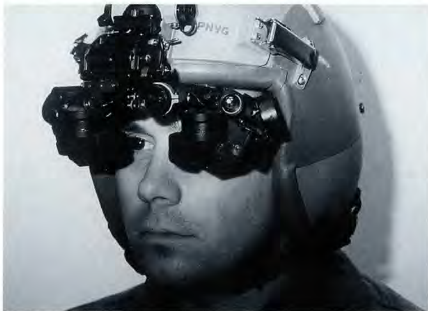
Armstrong Laboratory's Capt Robert T. MacMillan wears the prototype of the revolutionary Panoramic Night Vision Goggle that displays a 100-degree horizontal by 40-degree vertical, intensified, panoramic field-of-view, thereby increasing what the warfighter sees by 160 percent.
