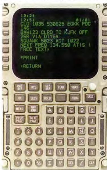
A typical ACARS control panel. Aircrews can request information and acknowledge receipt of information by use of subscriber designed codes.
