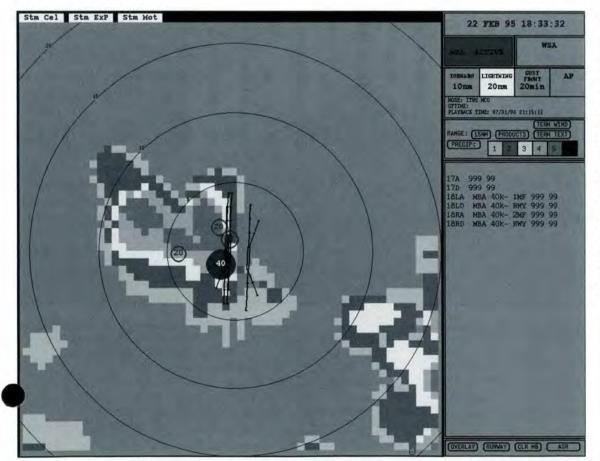
This is a display of the terminal doppler radar products as displayed in the air traffic control tower. The 40-knot circle indicates a microburst of a 40-knot loss of air speed. This is the product the air traffic controller will use.
