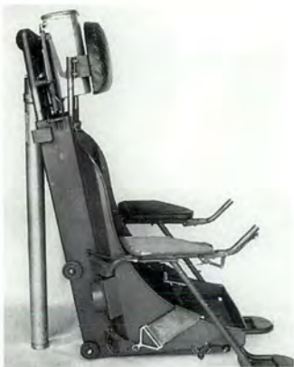
Above: An early prototype seat for use in the F-80. Right: Ejection seat used in later F-84s and the F-105.
