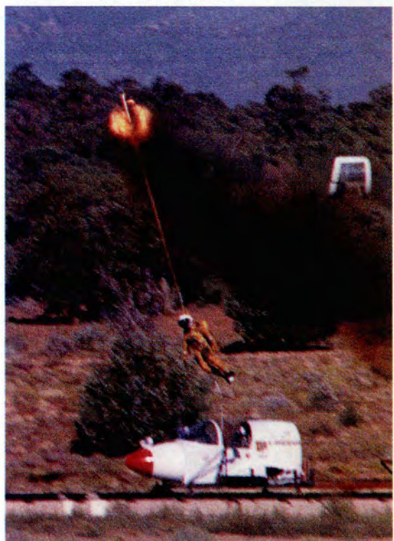
Below: Testing the RANGER extraction system, similar to the YANKEE system used on A-1 Skyraiders in Vietnam.
