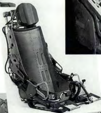
Above: An early prototype seat for use in the F-80. Right: Ejection seat used in later F-84s and the F-105.
