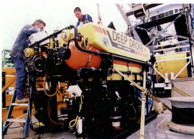
The US Navy's Remotely Operated Vehicle (ROV) Deep Drone is prepared before one of its 30 dives in water as deep as 5000 ft. In all, the ROV logged 244.5 hours of dive time recovering wreckage from King 56.
