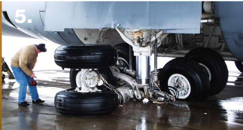
in and day out, in flight or parked. They include stresses to support aircraft weight while parked, stresses due to internal nitrogen pressure, and residual stresses created during initial manufacturing or operational damage. Because landing gear structures support aircraft weight most of the time, they are SCC factories!
