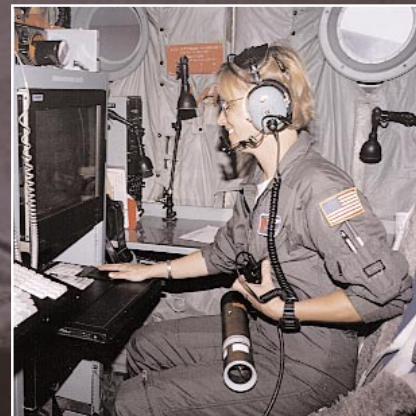
SSgt Kari Kennedy preprograms tracking information prior to releasing a dropsonde into the hurricane.
