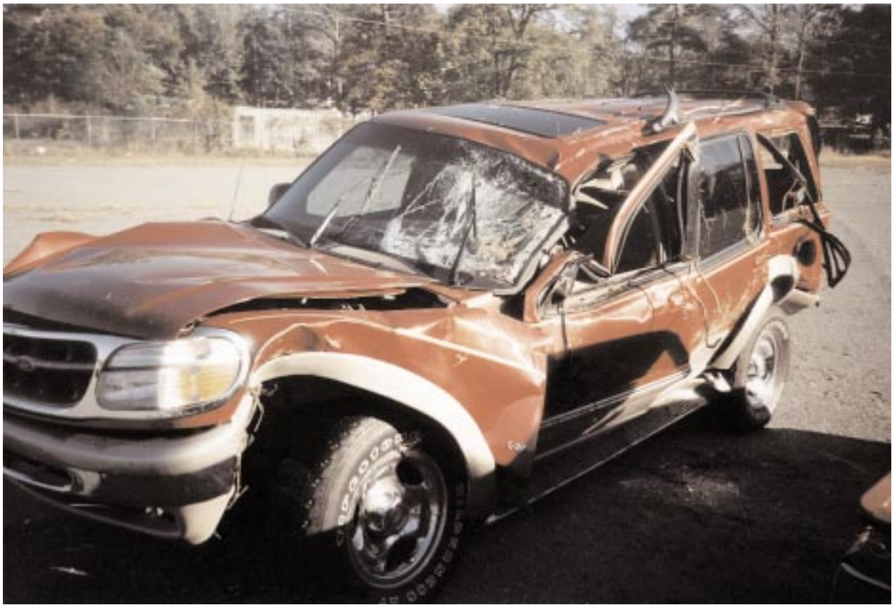
▲ The damage suffered by the Ford Explorer clearly indicated that it had rolled side-over-side as it went down the embankment. ▼
