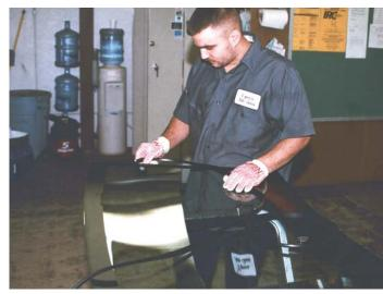
Wearing gloves while working around the edges of a windshield prevents oils from the repairman's fingers from getting on the glass and weakening the seal.
