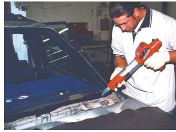
Properly applying the windshield adhesive is essential to getting a good seal. Poorly applied adhesive can allow the windshield to pop out during a collision.
