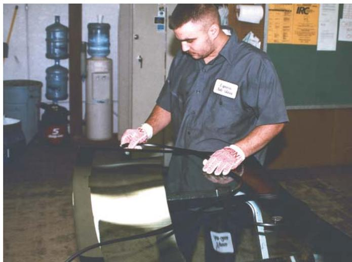
Wearing gloves while working around the edges of a windshield prevents oils from the repairman's fingers from getting on the glass and weakening the seal.
