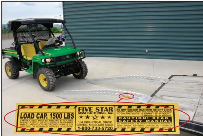
Figure 30—Load capacity rating for a ramp.
