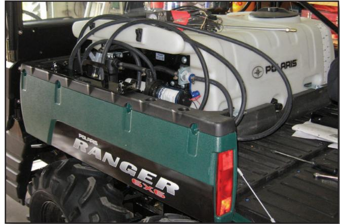
Figure 55—UTV being equipped with a pesticide sprayer. Courtesy of Jim Goodwin.
