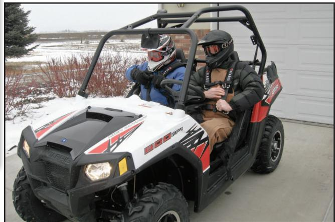
Figure 40—An operator and passenger make sure their seatbelts are fastened securely. Courtesy of Michael Donch.
