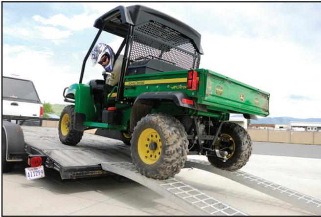
Figure 35—An operator slowly unloads a UTV while ensuring the wheels remain centered on the ramps.
