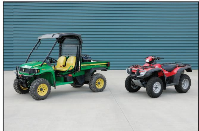
Figure 9—UTV (left) and ATV (right).
