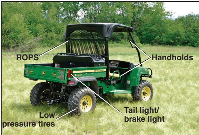
Figure 8—Features of a UTV (rear view).
