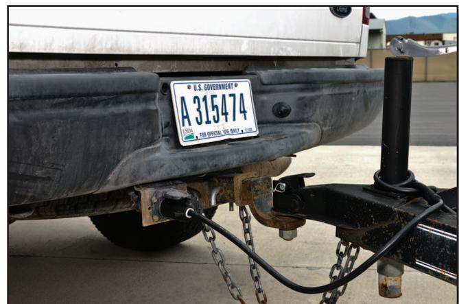
Figure 29—A trailer correctly hooked to the towing vehicle.
