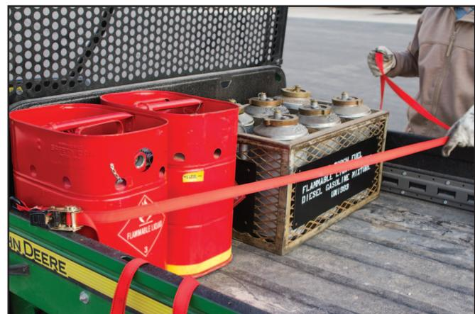
Figure 38—An employee secures cargo with a tiedown strap.
