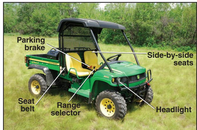
Figure 7—Features of a UTV (front view).
