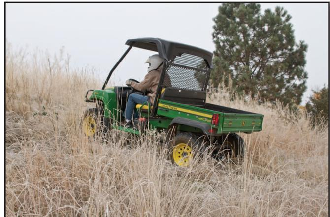
Figure 48—An operator climbs straight up a slope.
