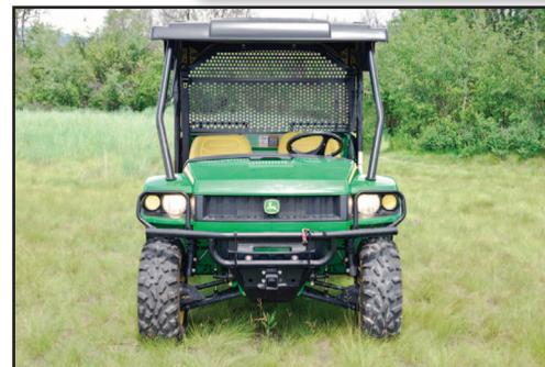
Figure 25—Operational lights on a UTV.
