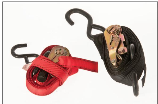
Figure 34—Ratchet-type tiedowns are used to secure UTVs to a trailer.
