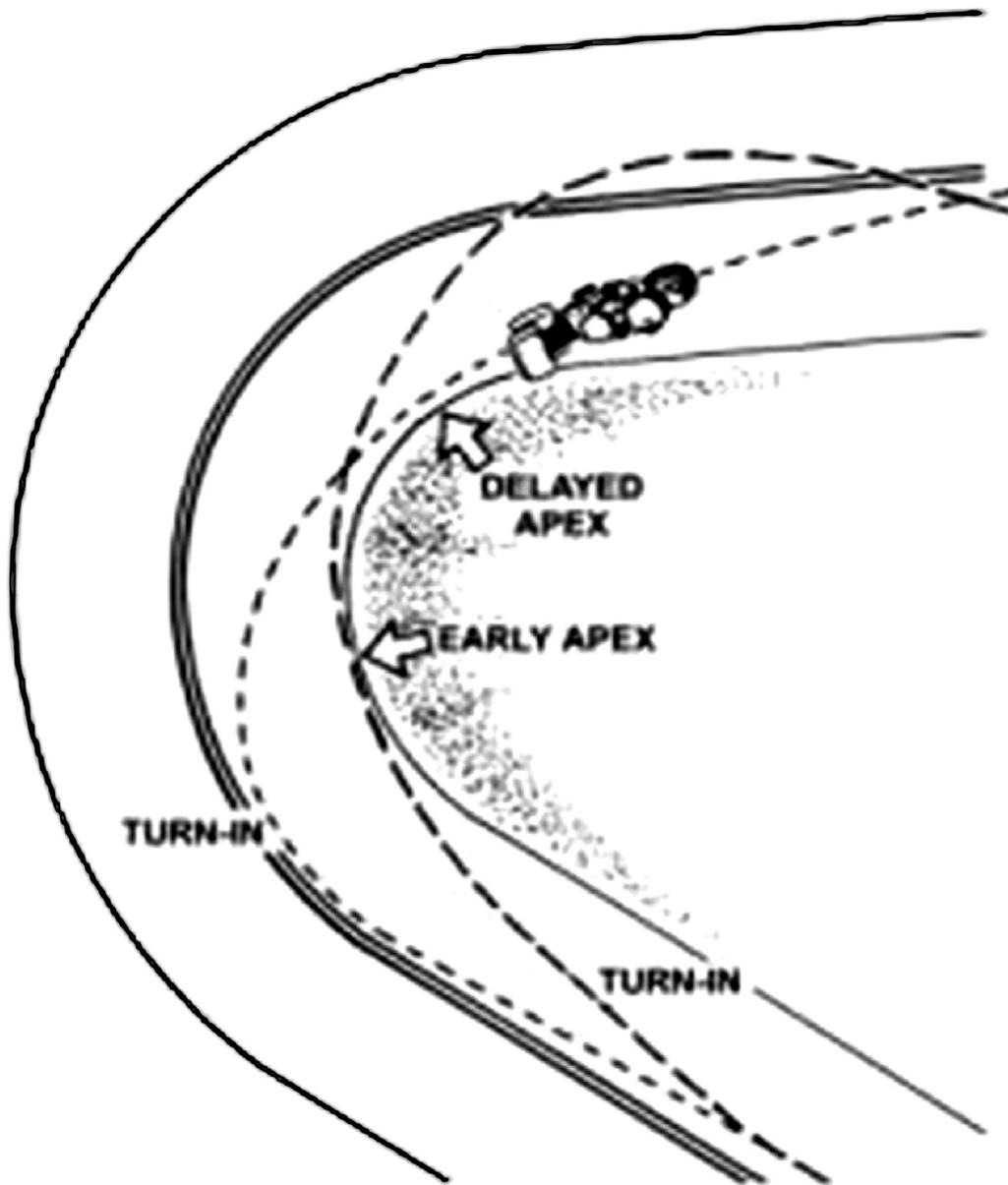
**Figure 2.** Delayed apex on a decreasing radius turn
