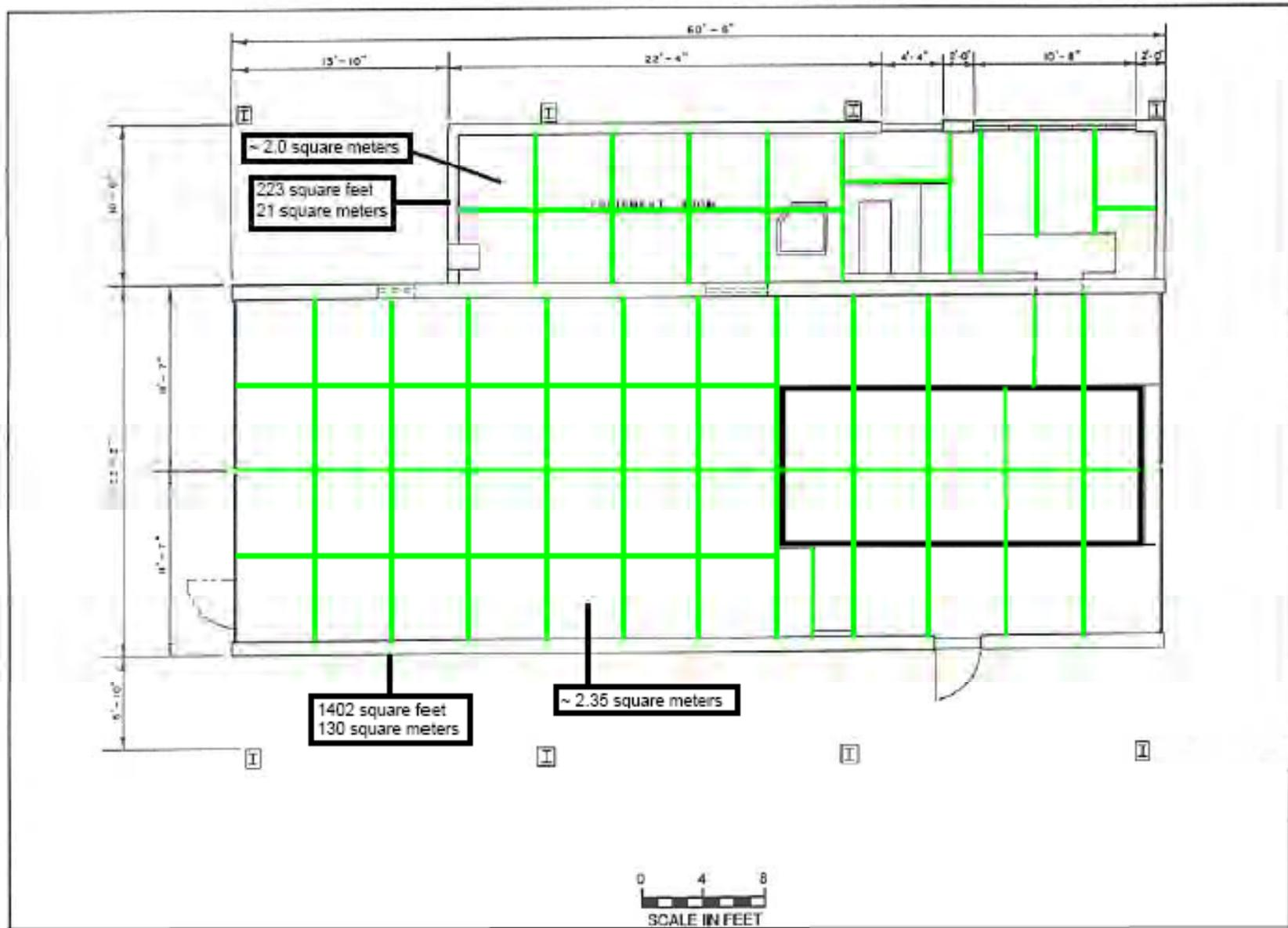
Figure D-2. Example Grid System for Shelter Floor and Pit Surveys.
