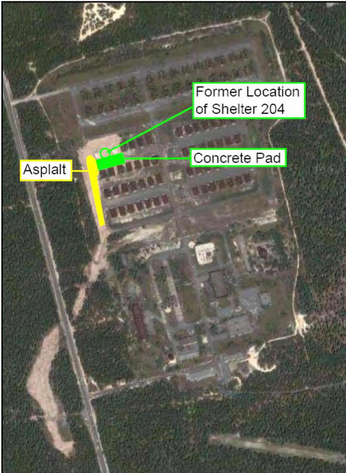
Figure A-4. Aerial Photograph of the BOMARC Site Indicating Areas Where Concrete and Asphalt were Poured.
