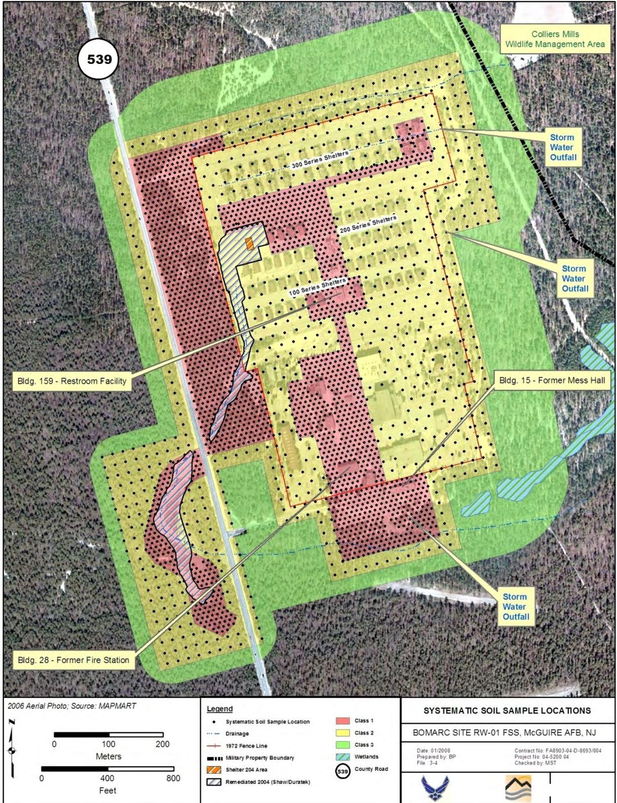
Figure C-15. Systematic Soil Sampling Locations Supporting Final Status Surveys in Secondary Areas (Cabrera 2008).
