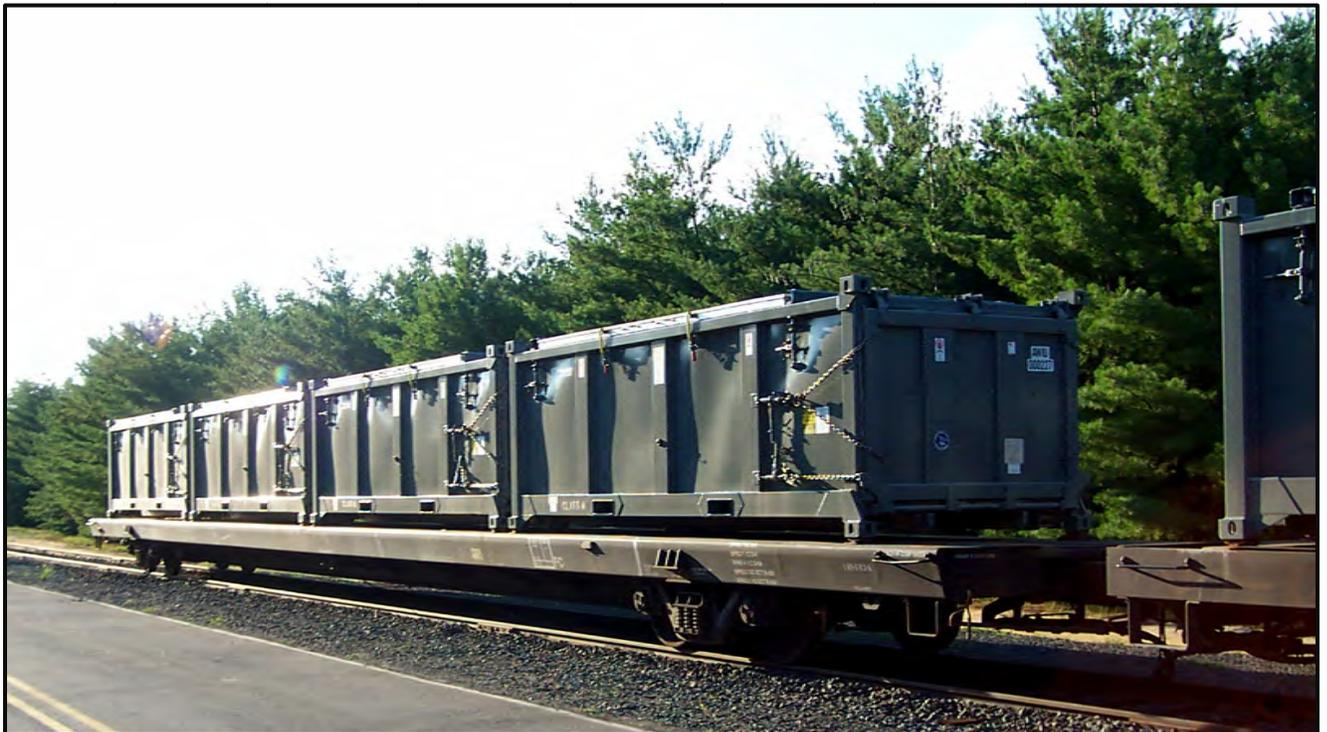
Figure B-3. Flatbed Rail Car used to Carry Four Intermodal Containers.
